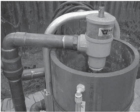
Figure 9a: Typical Cleanable Flush Cart Strainer (100 mesh [0.149mm])
